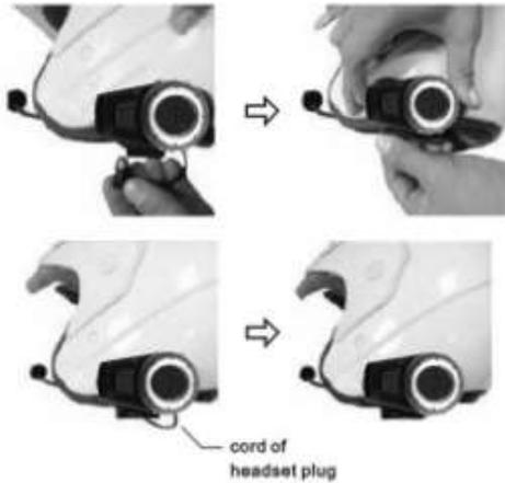
4. Taking care to match the pins up, connect the Headset Plug to the Headset Socket. The plug can only be inserted in one position.
