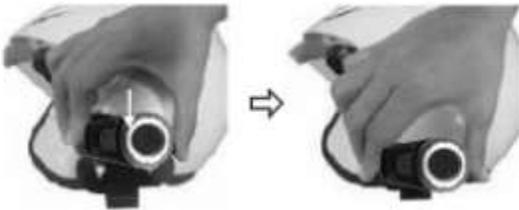
2. Now you need to attach the speaker and microphone arm to the inside of the helmet. Take the Velcro pad which the speaker will attach to, and test for the best position to fix it. The Velcro Pad should be fixed at the height of your ear in the helmets ear pocket. You will need to put the helmet on a few times to find the optimum position to apply the pad. When the correct positioning is found, remove the protective strip and apply the Velcro Pad.
