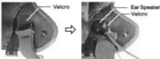
3. Next, take the Ear Speaker and attach it to the Velcro Pad. Run the Microphone Arm down along down to where your mouth will be. As the Microphone Arm is flexible, you can adjust it so it sits in the optimum position in front of your mouth. Some helmets have removable padding; if yours does, it is recommended to run the speaker and microphone under the padding.
