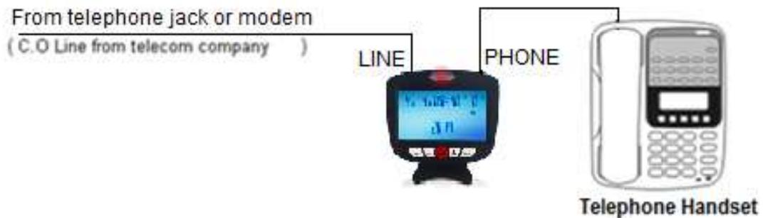
PARALLEL (Option 2): You may also install it in parallel with your phone(s) using a 2-way splitter (not included), as shown below:
