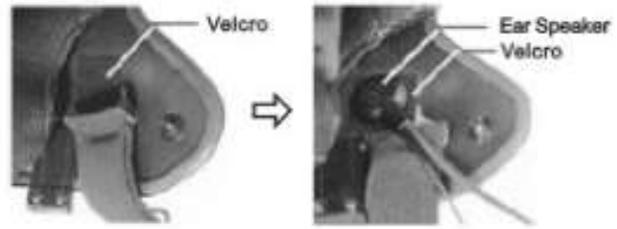
The Velcro pad should be fixed at the height of your ear in the helmet's ear pocket. You will need to put the helmet on a few times to find the optimum position to apply the pad. When the correct positioning is found, remove the protective strip and apply the Velcro Pad.
