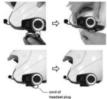
5. Secure the cord of the Headset's plug inside the helmet. Tuck any extra wire into the helmet. Try to hide the cable as much as possible under the padding. Now you have successfully mounted the Headset on your helmet.
